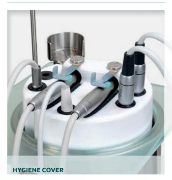
For regular cleaning of the water lines, the instrument hoses are simply inserted into the hygiene cover. With the command "Normal flushing" the instruments are flushed in accordance with RKI after 120 seconds. After prolonged periods of inactivity, the "Intensive flushing" function ensures perfect water quality.
